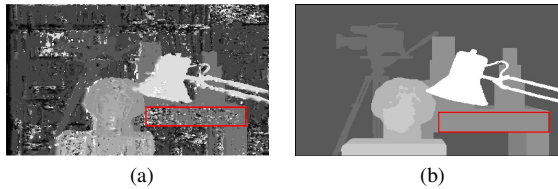
Fig. 1: Disparity maps: (a) a raw map and (b) a ground truth map.
